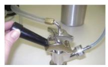
STEP 7 After the tap tower has been placed on the refrigerator and the hose line feeds through the bottom, attach the wing nut to the coupler.
